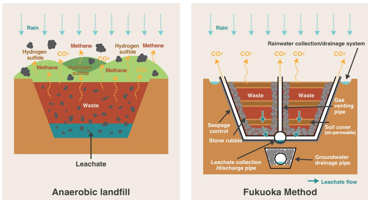
Fig. 2 Structural diagrams of Fukuoka method and anaerobic landfill method (created by Fukuoka Prefecture)
