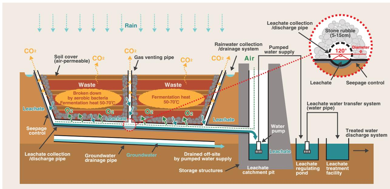
Fig. 1 Structural diagram of Fukuoka method for final waste disposal sites (created by Fukuoka Prefecture)
