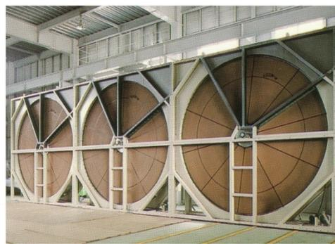
▲ VOC concentrated rotor. Hydrophobic zeolite supports inorganic honeycomb.
